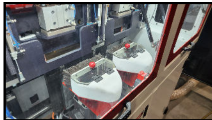
Servo Positioning Of Cutter Heads
