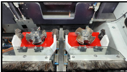
Counter-Rotating Cutter Heads
