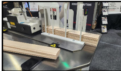
Material Hopper Feed System
