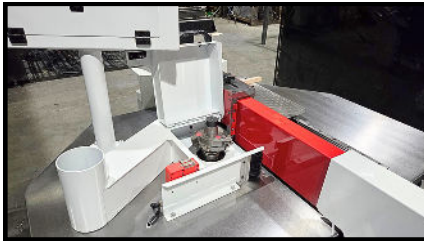
Single-Spindle HSK Setup
